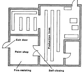
Fig. 3 Layoctmodetmyptcal Engineettingdd/cerkshop, showing compartmentation/segregation of a hazardous area like paint shop.
