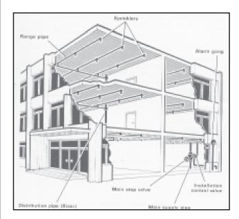
Fig-20. Layout of a typical Sprinkler Installation
