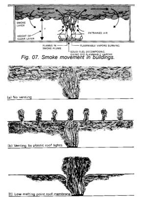
Fig. 08. Effect of venting on flames beneath a ceiling.
