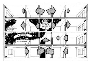
Fig. 2 Smoke Movement and Stack Effect in a Multi-Storey Building.
