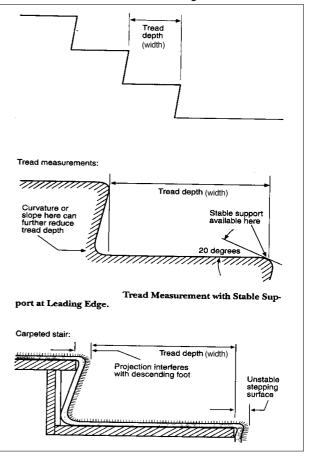
Fig. 16 . Measurement of Tread depth (width)
