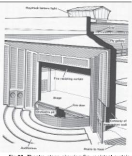
Fig-22. Theatre stage showing fire resistant curtain and proscenium wall
